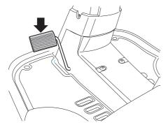
The blade drive is not affected by the clutch pedal.
